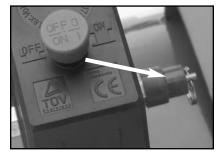
Figure 8. Safety drain valve.
